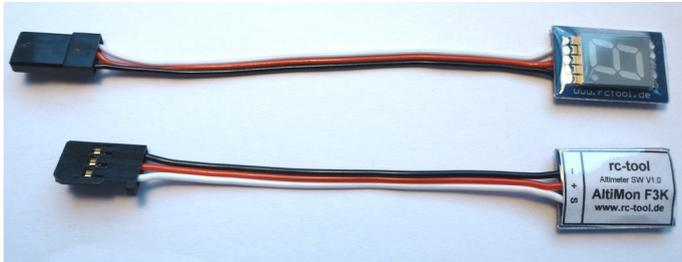
After landing the maximum reached altitude of the last flight can be read from the 7-segment display. An undervoltage detection warns the pilot before the battery gets empty.
